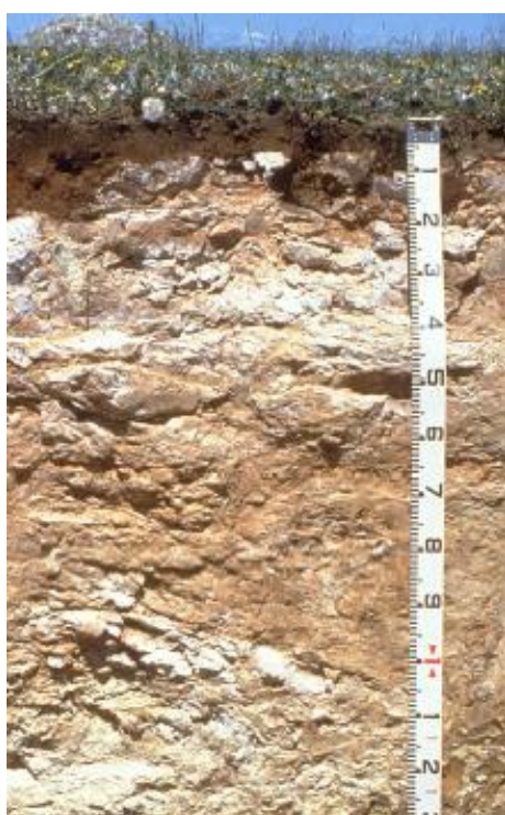
Large fragments of calcrete in this soil profile result in very low waterholding capacity
