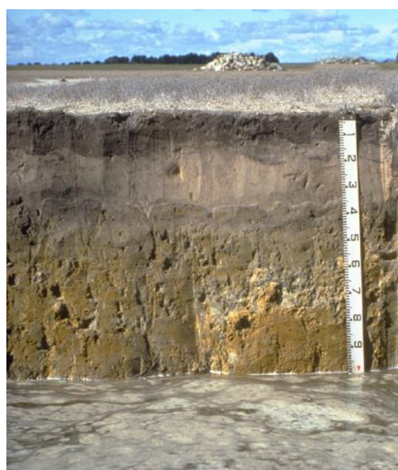
Groundwater within ~200 cm depth can rise by capillary action, bringing moisture (and often salt) into the plant rootzone and surface soil
