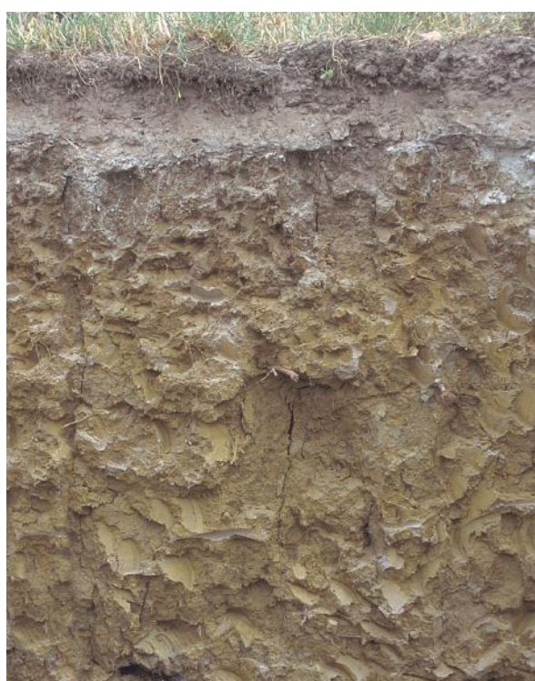
Sandy loam over poorly structured heavy clay subsoil
