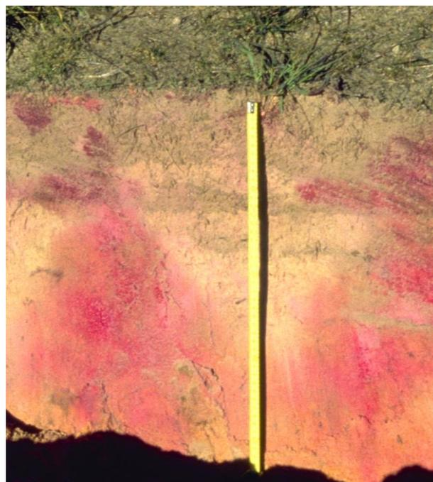
*Pink dye applied uniformly at the surface shows uneven wetting patterns in a water repellent sand*
