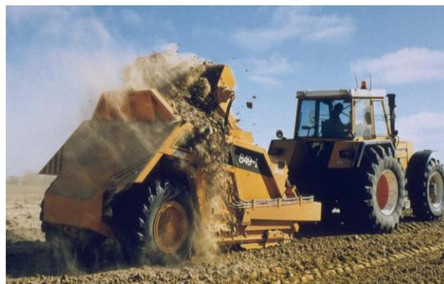
Clay spreading to ameliorate water repellence
