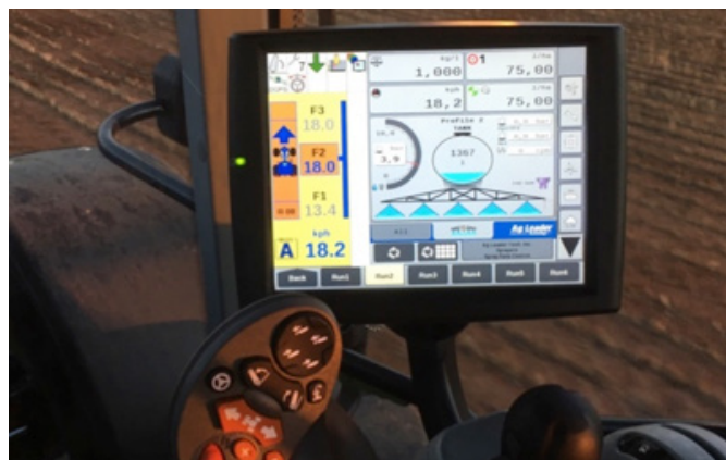
Spraying monitor with auto section in operation.
