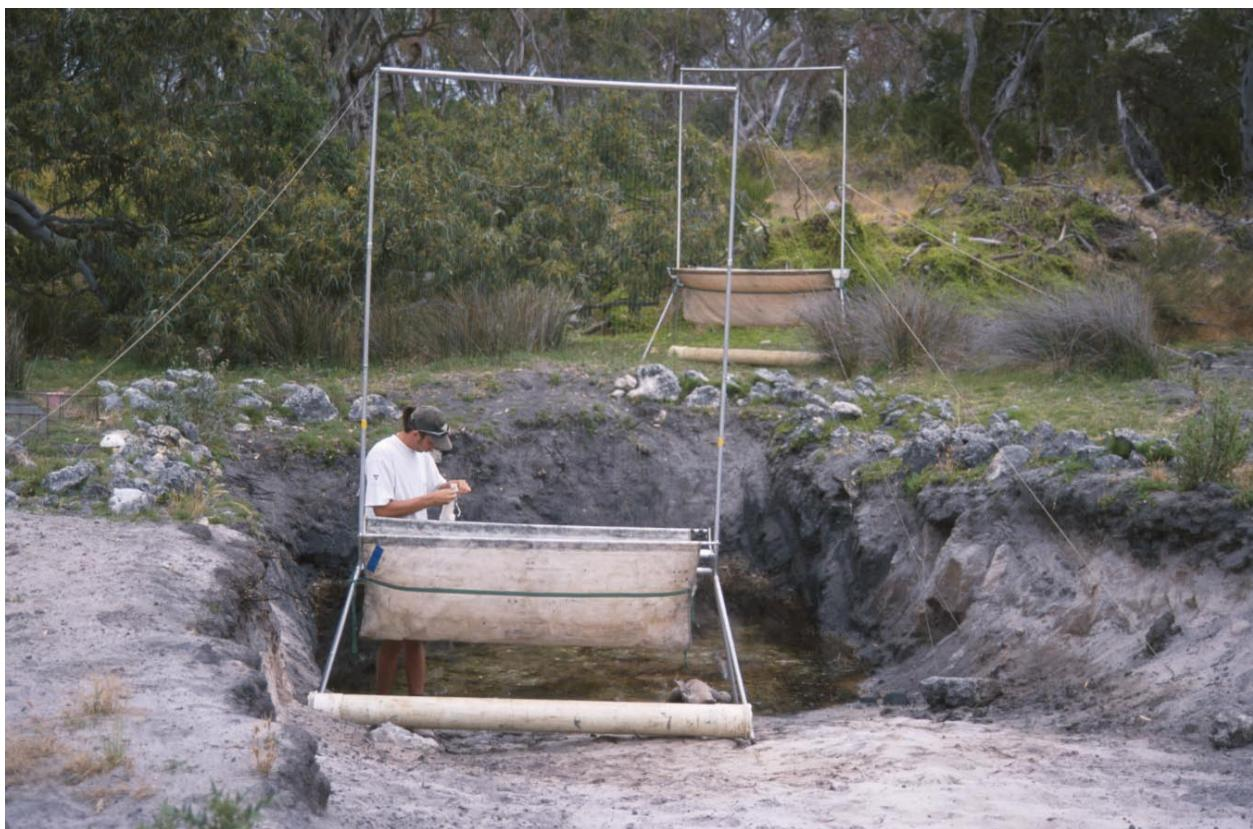
**Figure 3. Andrew Freeman checking Harp Traps, which were used to capture bats during the Biological Survey of the West Avenue Range, December 1999.**
