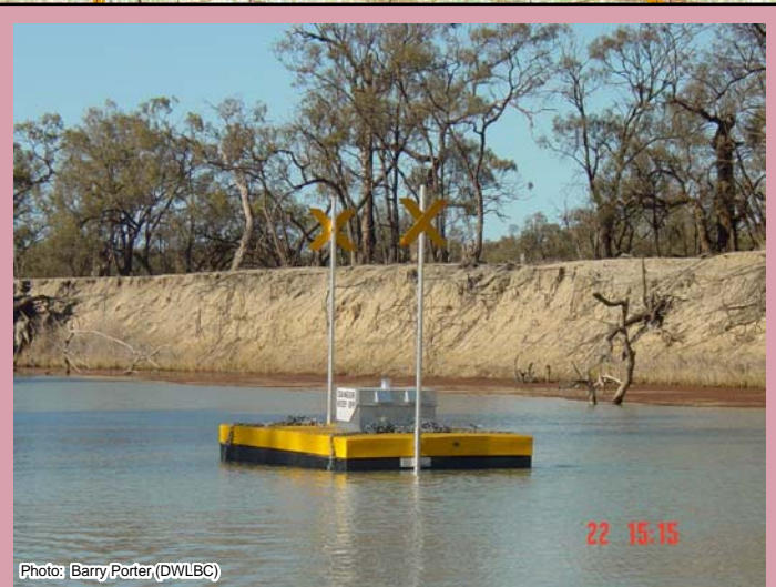
Continuous flow and salinity recorder mounted on pontoon at Lettons
