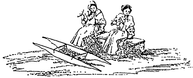
Figure 5. "Bal Maidens" clobbering or bucking ore, breaking up the large lumps for sorting. Mid 19th Century Cornish.
