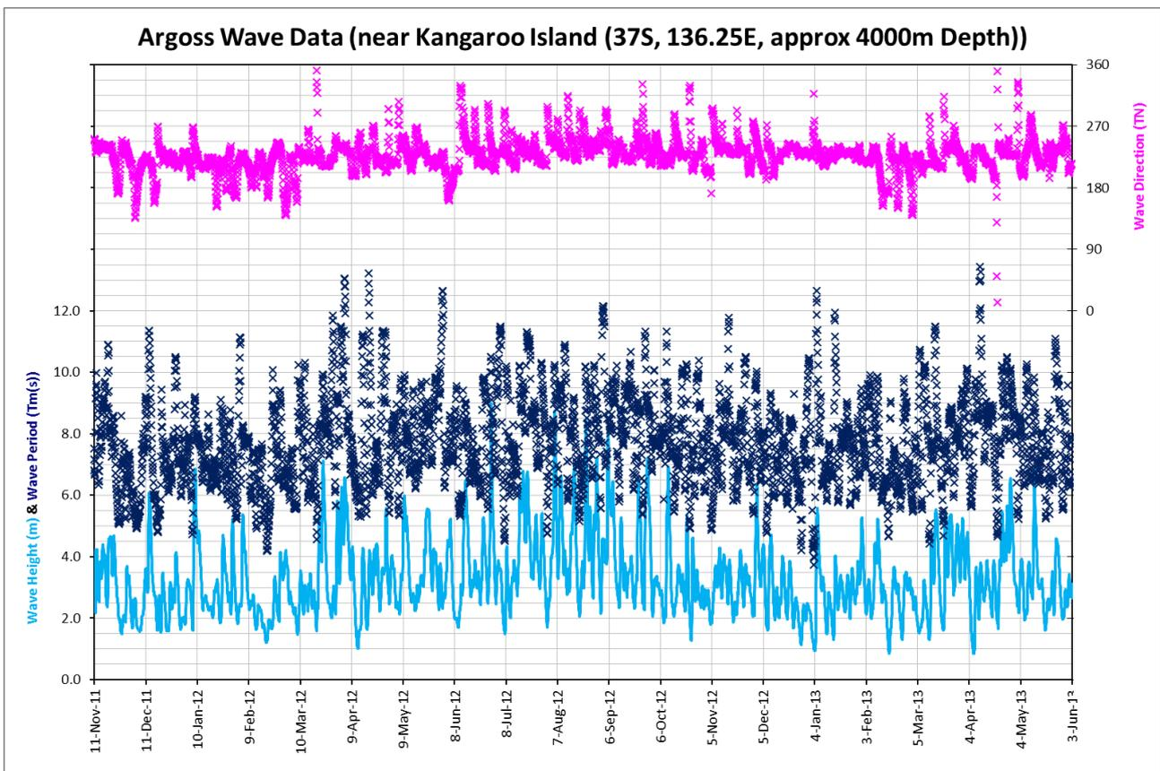
Figure 3-14 Offshore Wave Height, Period and Direction Timeseries
