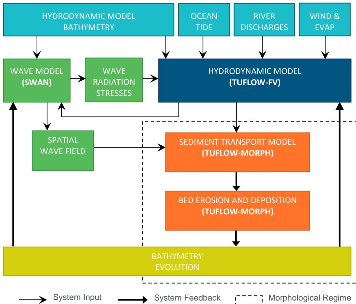
Figure 3-3 Interactions between Hydrodynamic, Wave and Sediment Transport Models
